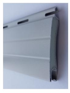
Slats are double walled cavity, curved profile with a Polyurethane foam for added strength and insulation.
